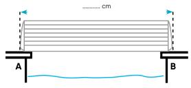
Min. distance between casing = pool width [AB] + 55 cm
